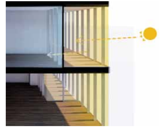
Double Thermal Barrier (North)
