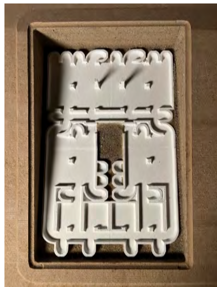
SYSTEM MODELED 1/16":1' MODEL WITH REMOVABLE FLOORS AND LIGHTING
